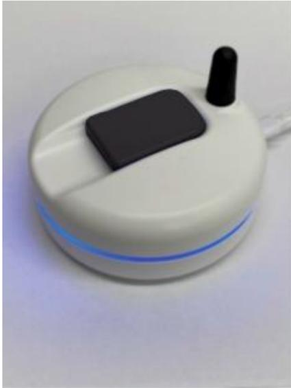
The CADI Optimum AIR Docking Station when plugged in will flash blue two or three times before going dark.
